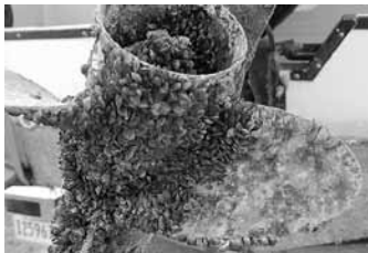
Quagga mussels on a boat propeller. Aquatic invasive species can clog water-intake structures, such as irrigation pipes. Photo credit: National Park Service
